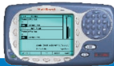
RTU with optional display running pump controller module
